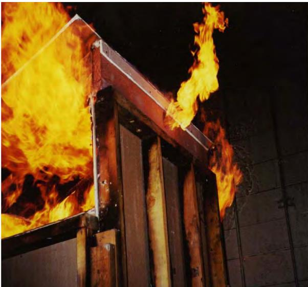
**Flame intrusion into attic through a vent**
